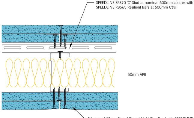
2 layers of 15mm Knauf Soundshield Plus fixed with SPEEDLINE Drywall Screws at 300mm centres (200mm centres at external angles). Ref to table for fixing length.
